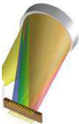
Figure 14 Grating and diode array
